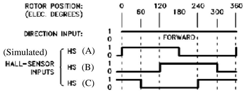
Fig. 2 – 6-Step Commutation timing
