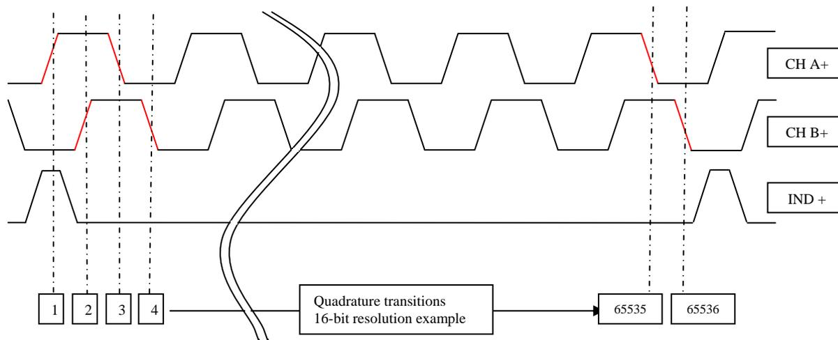
FIG A: Encoder Resolution / Quadrature Transition Relationship
