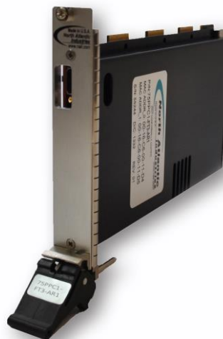
NAI 75PPC1-FT3-AR1 Single Board Computer
