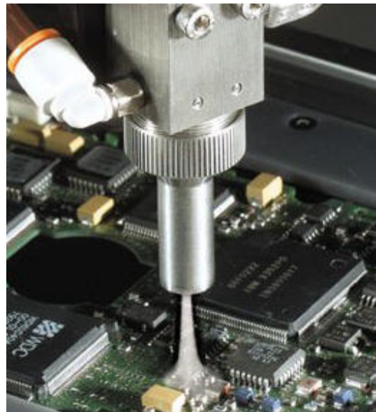
Fig 1. – Robotic Selective Coating Systems, such as the system used by NAI, provide the highest quality conformal coating available.
