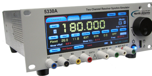
NAI's 5330A is the latest in Digital Synchro/Resolver Simulation technology. Intelligent DSP design allows all programming via touch-screen or mouse interface.
