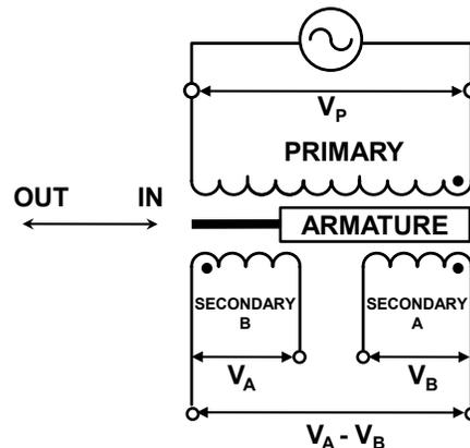
Fig. 2 – Elements of an LVDT.
