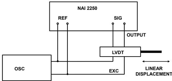
Figure 5 – Test system connections.
