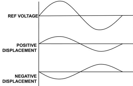
Figure 3 – AC signal from LVDT
