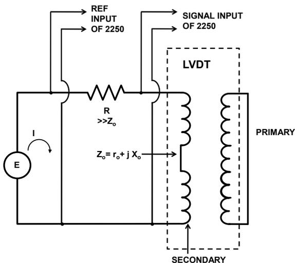
Figure 8 – Measurement of the output impedance
