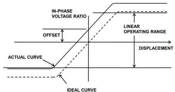
Figure 6 – Offset can be eliminated either manually or by computer.
