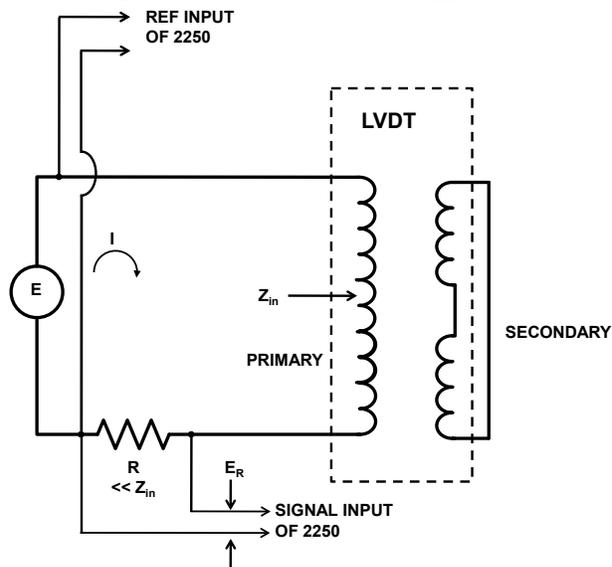
Figure 7 – Measurement of the input complex impedance of the primary winding.
