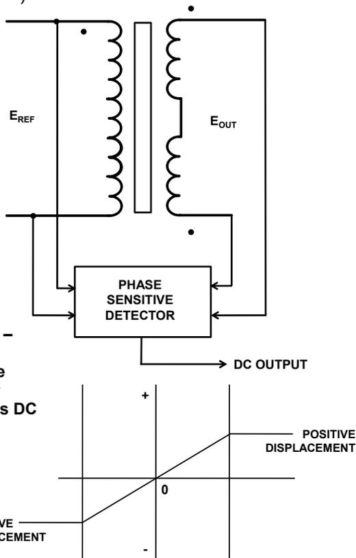
Figure 4 – Phase-sensitive detector produces DC output
