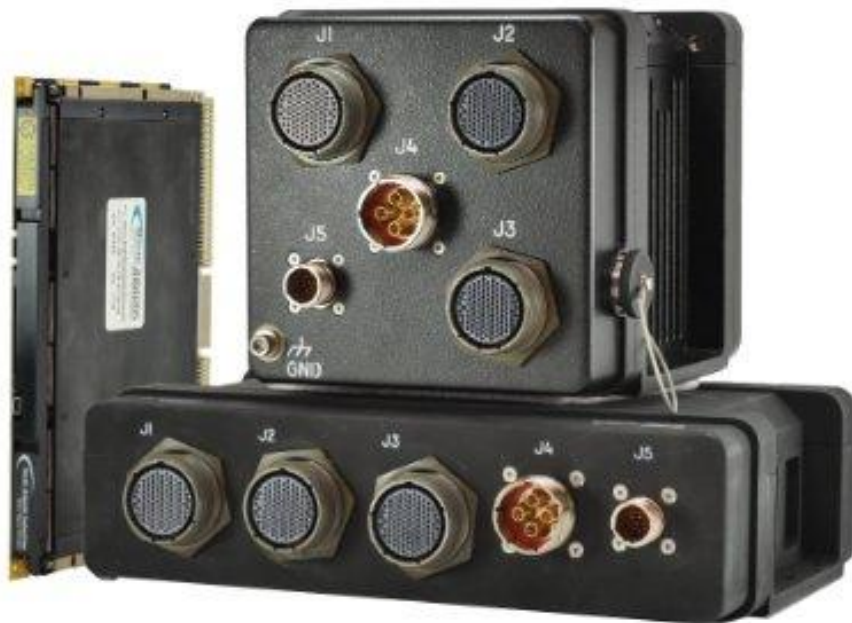
Figure 3: Common platform/distributed Discrete I/O
